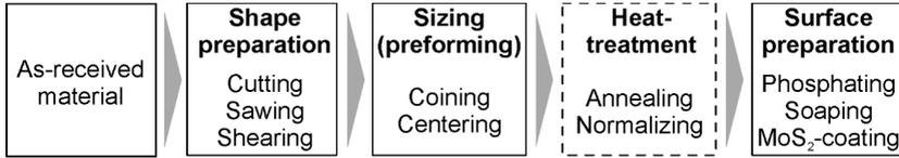
**Figure 2.17:** Billet preparation steps in cold forging (based on Lange et al., 2008)
