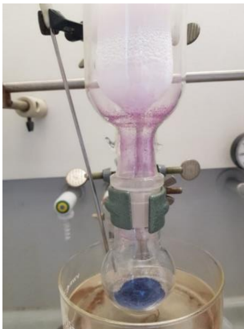
Figure S7: Sublimation setup for the removal of excess acetamide from crude [\text{Rh}_2(\text{acam})_4] ( 10 ). The sublimed acetamide is caught on a cooling finger filled with a dry ice acetone mixture at -78\text{ }^\circ\text{C} . The remaining blue solid is [\text{Rh}_2(\text{acam})_4] ( 10 ).
