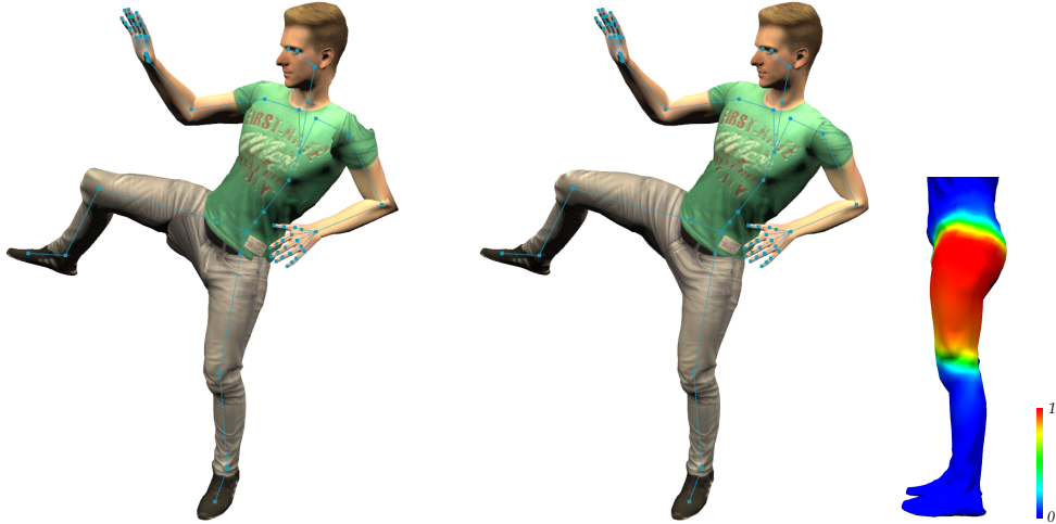
Figure 2.2: Assigning each skin vertex to a single joint results in a rigid, block-like skinning (left). Blending multiple transformations allows for smoother transitions at joints (Linear Blend Skinning, right). The character’s skinning weights that correspond to the hip bone are visualized on the right.
