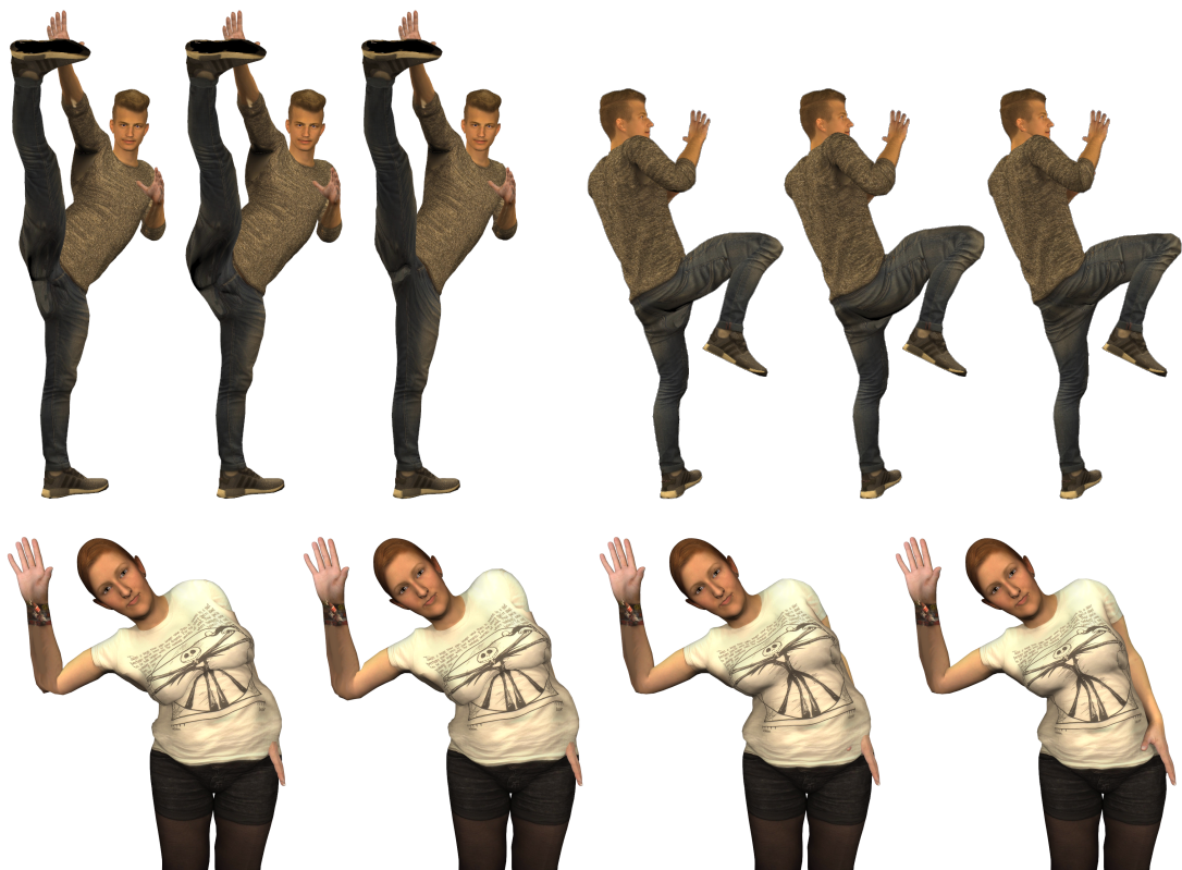
Figure 3.17: Three example poses. From left to right: Linear Blend Skinning, Dual Quaternion Skinning and our Fast Projective Skinning. The rightmost bottom image shows our FPS result with global collision handling enabled.
