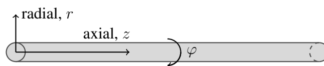
Figure 3.1: Coordinates, axial and radial direction along a cable.
