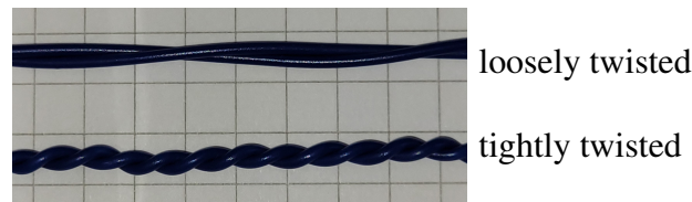
Figure 8.3: Photo of a section of the two twisted pair cables.
