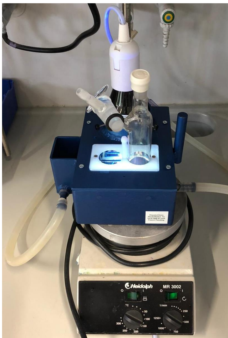
Figure S5. PhotoRedOxBox TC from Hepatochem.
