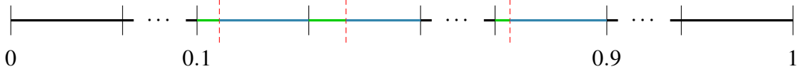
Figure 3.7: Modified model problem MP for numerical tests in one dimension: We consider the interval [0, 1] and between x = 0.1 and x = 0.9 we split every cell into a pair of two cut cells, which are marked in green and blue.
