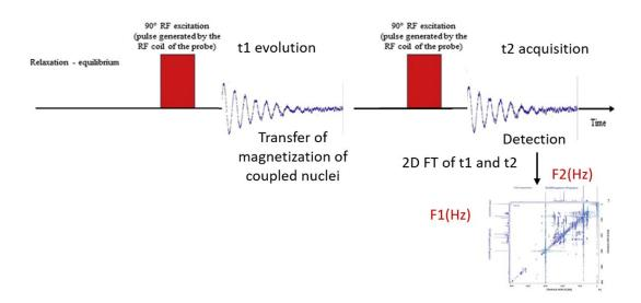
Figure 3.4: Two-Dimensional NMR spectroscopy pulse-acquisition. Adapted from [118]
