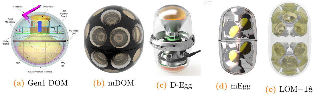
Figure 3.4: A schematic view of optical modules is shown. Gen1 DOMs [26] are used for the current IceCube detector, while mDOM [37] and D-Eggs [32] will be deployed in the IceCube-Upgrade; mEgg and LOM-18 are two of various potential designs for IceCube-Gen2 [38, 39]. Figure taken from Ref. [38].
