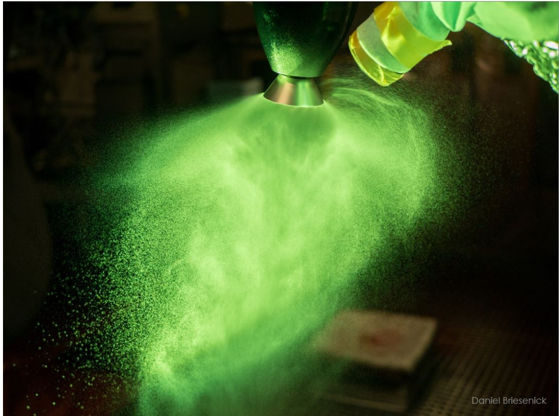
Figure 3.7: High-speed imaging with back-light laser illumination during atomization of clear coat - copyright by D. Briesenick, BASF Coatings GmbH.
