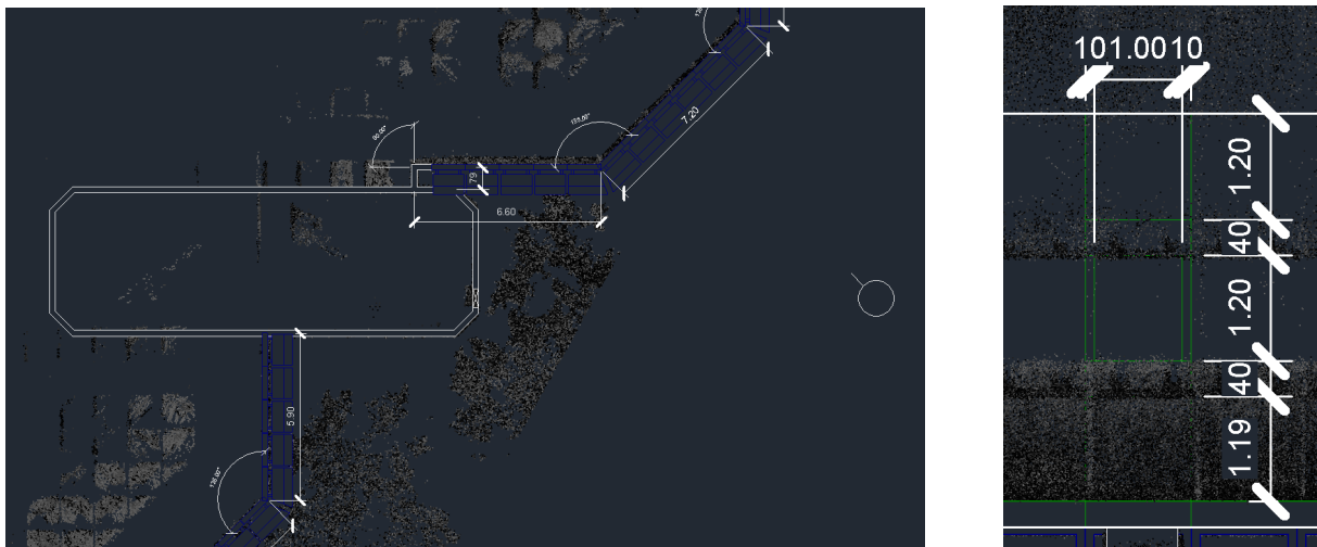
Figure 31: Floor Plan of Point Cloud/Walls with Measurements (left), Length Measurements of Windows (right) (own illustration)
