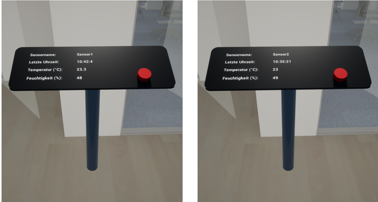
Figure 77: Button-Triggered Display of Sensor Values in the Running VR Application (own illustration)
