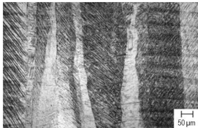
Figure 2.2: Anisotropic microstructure in a SLM part made of titanium [28].
