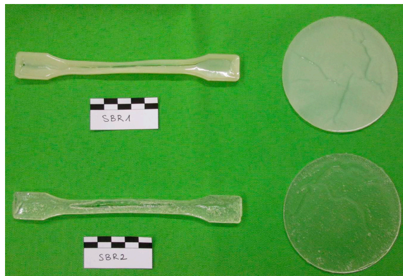
Figure 1. Overview image of the synthesized round and dog bone samples SBR1 and SBR2. The dog-bone samples are 170 mm long; the diameter of the round samples is 90 mm.
