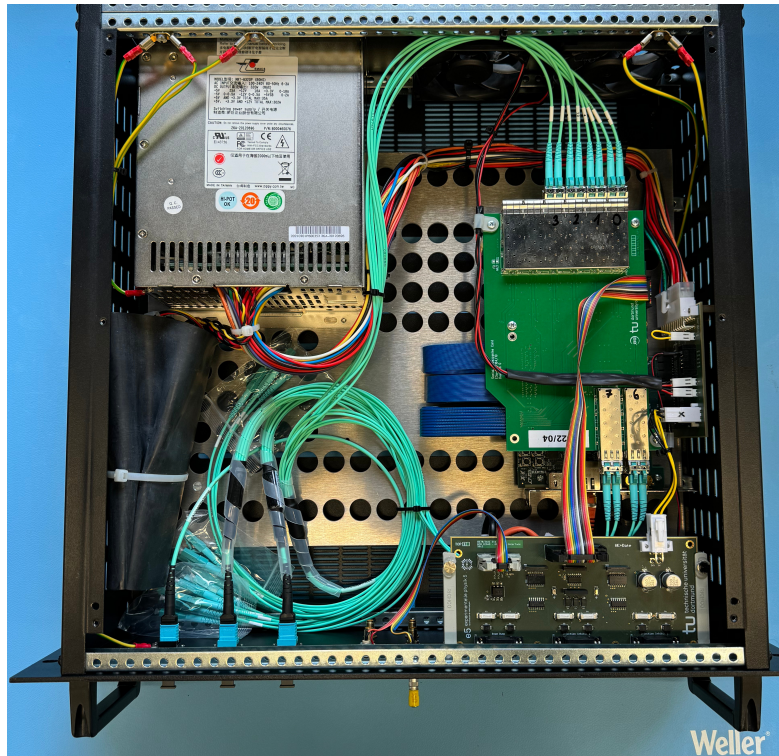
Figure 6.1.: Bird's-eye view of the MIBAD crate without fiber optic cables and XCVRs installed. Mounted on the baseplate on the right-hand side is the main FPGA board, which is mostly covered by the optical mezzanine card. The interface signals are routed via the BCM mezzanine to connectors on the front plate. Power is supplied via the redundant power supply located in the top-left corner of the crate.
