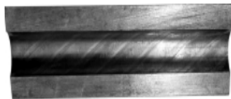
Figure 2: Effect of spiralling on the bore hole wall
