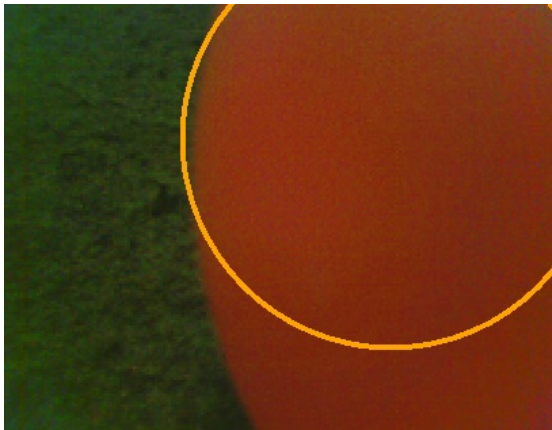
(a) A falsely recognized ball. The ball is too dark for a correct detection with an approach using only a single standard color table.
