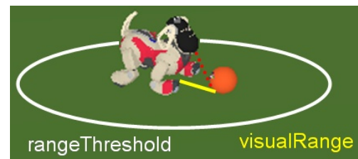
(b) Since the visualRange is smaller than the rangeThreshold , the nearColorTable is used.
