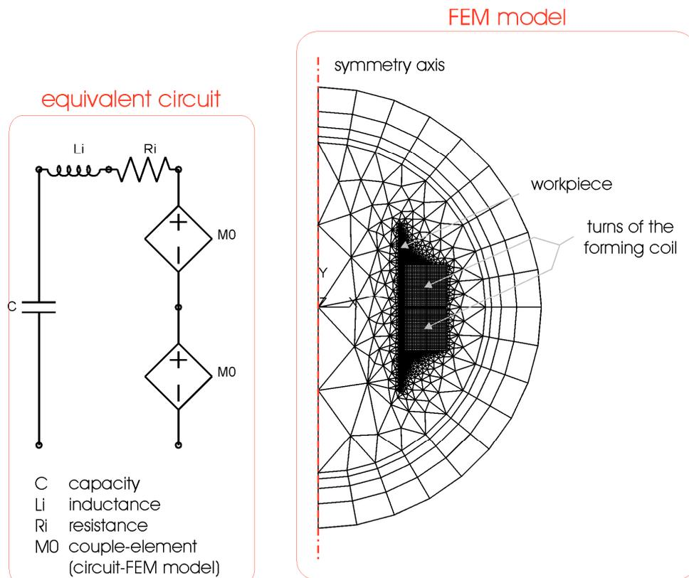
**Figure 2:** Coupling between equivalent circuit and FEM model
