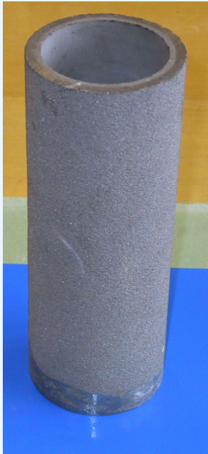
Multilayer element made of titan powder. \text{Ø} = 40 \text{ mm} , H = 125 \text{ mm} .
