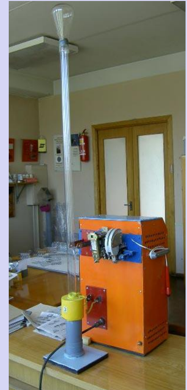
Conveying of powders and powder parts by pulsed electromagnetic field (Riga, RTU)
