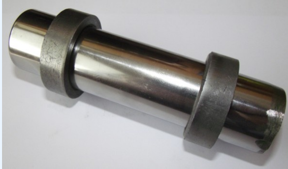
Powder parts on the steel mandrel
