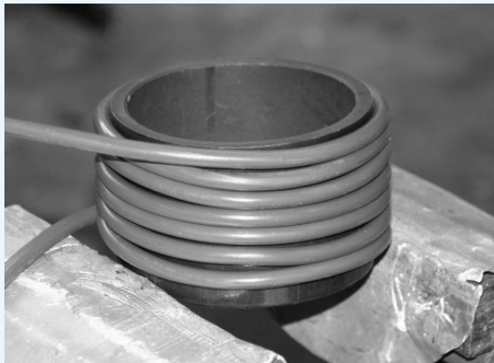
Single-action copper coil with powder parts inside
