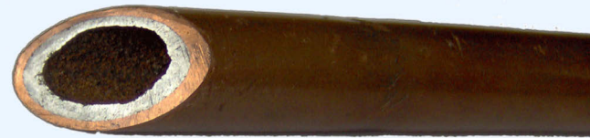
Permeable elements made of iron powder in copper shell. \text{Ø} = 10\text{-}40 \text{ mm} , H = 30\text{-}160 \text{ mm} .
