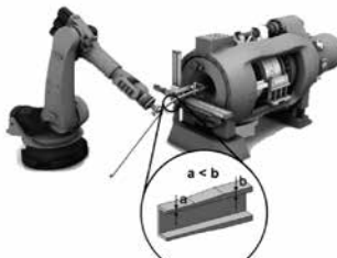
Direct hot extrusion
