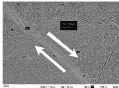
Left: Simulation result cutting process (material DP1000), right: Shear band formation in a Ti-10V-2Fe-3Al alloy (testing stopped at 10 % strain applied)/Images on the right by S. Winter (TU Chemnitz)
