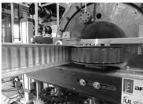
Hot extrusion and corrugation
