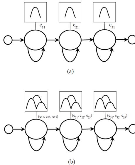
Figure 2.1: (a) A single mixture per state HMM and (b) A multiple (three) mixture components per state HMM;  $c_{jm}$  denotes the mixture weight for the  $m^{\text{th}}$  mixture of the  $j^{\text{th}}$  state.
