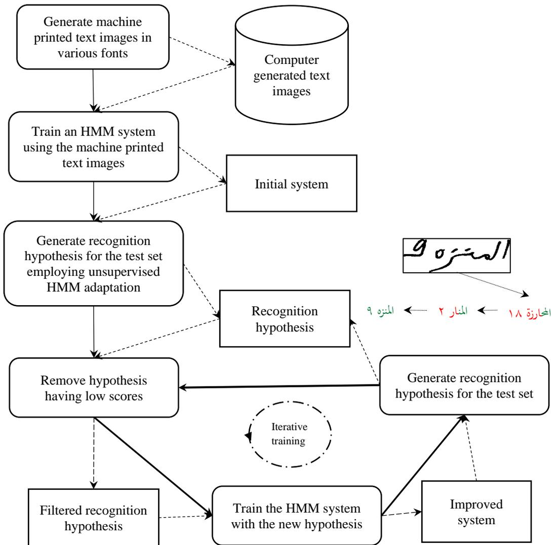
Figure 6.5: The process framework for Arabic text recognition without handwritten training set. (Handwritten text image source: IFN/ENIT (Pechwitz et al. 2002)).
