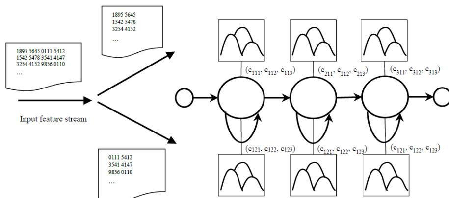
Figure 2.3: An illustration of multi-stream HMMs. The original feature vector split into two streams.  $c_{j^s m}$  denotes weight for the  $m^{\text{th}}$  mixture component of  $s^{\text{th}}$  stream of  $j^{\text{th}}$  state.
