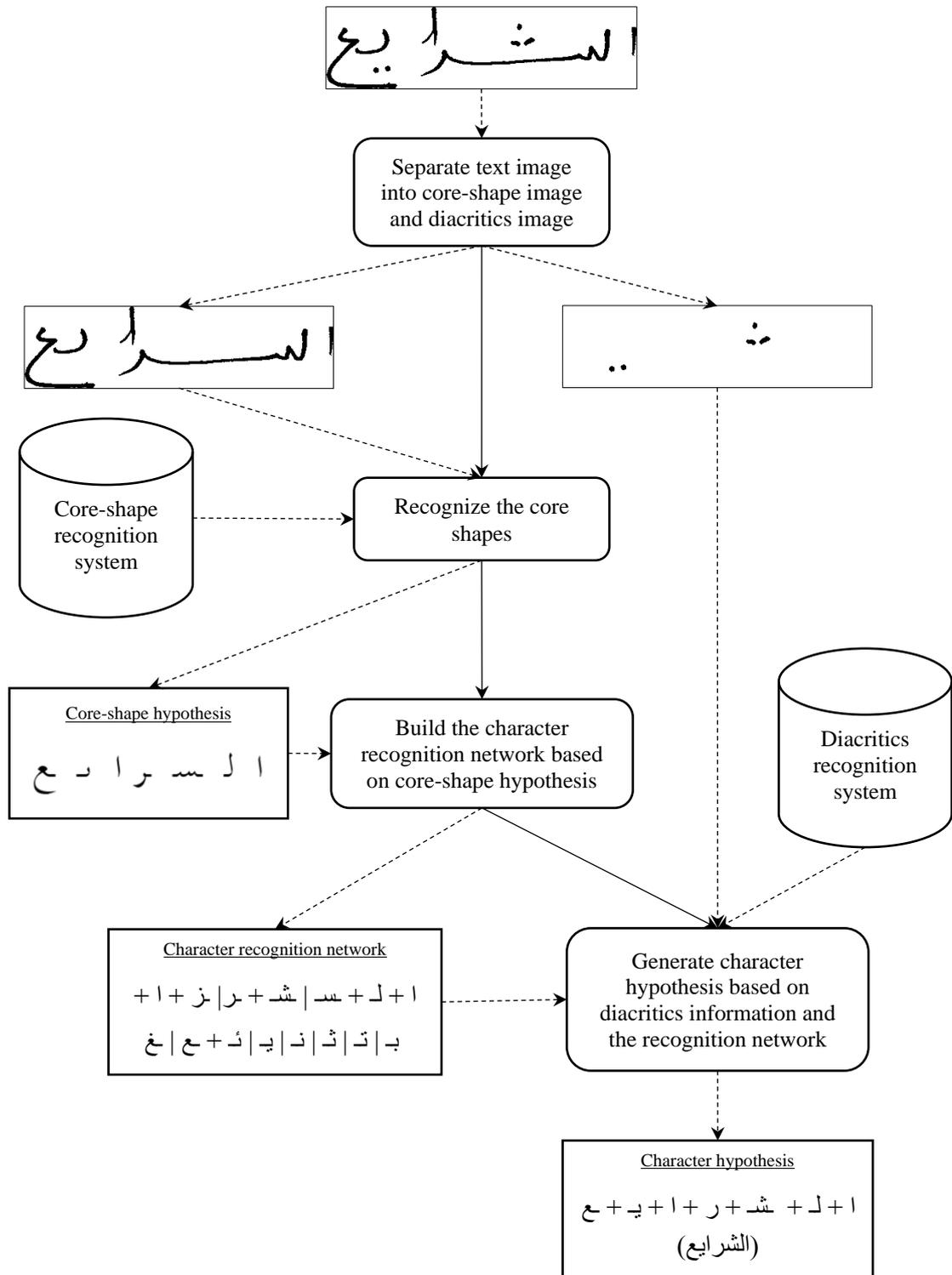
Figure 5.12: The multi-stage character recognition framework. (Handwritten text image source: IFN/ENIT (Pechwitz et al. 2002)).
