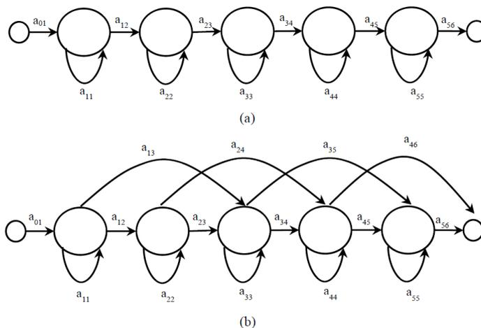
Figure 2.2: Two common HMM topologies used in text recognition; (a) A left-to-right linear topology and (b) A left-to-Right Bakis topology.  $a_{ij}$  denotes the state-transition probability from state  $i$  to state  $j$ .
