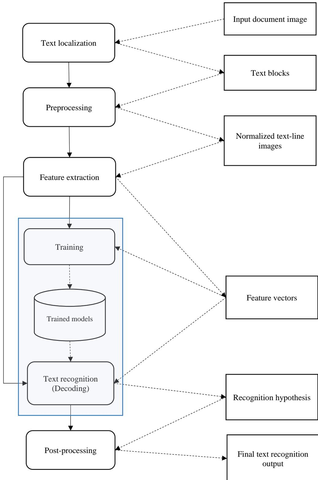
Figure 1.1: Process framework for a typical text recognition system. The shaded area shows the main focus and the scope of the present thesis.
