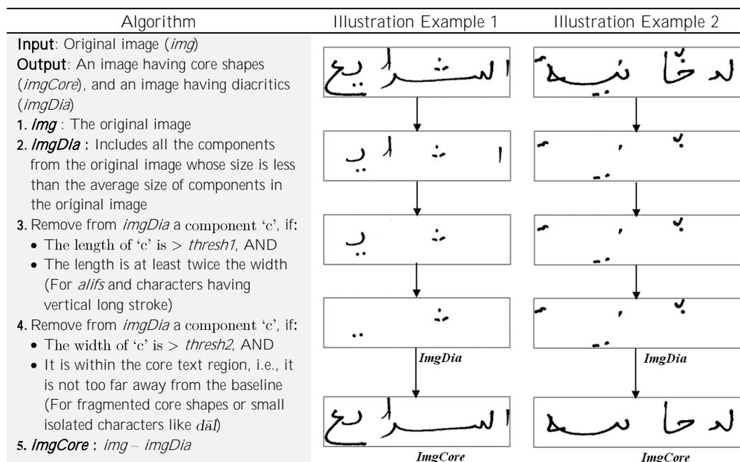
Figure 5.11: Core shapes and diacritics separation algorithm. (Figure adapted from (Ahmad and Fink 2015a))
