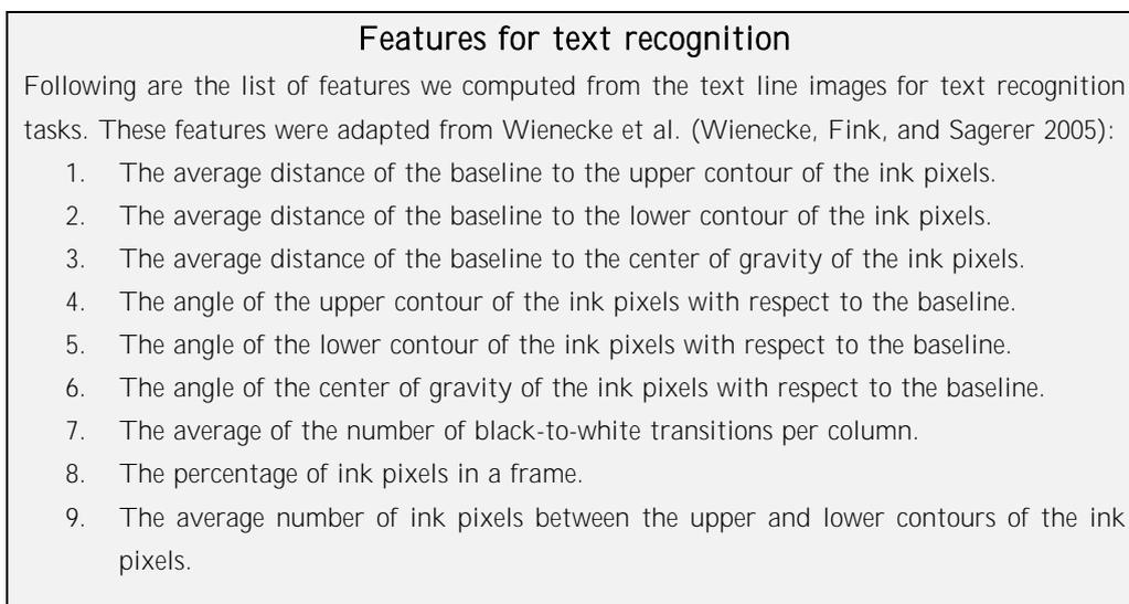
Figure 7.3: The list of features extracted from the text line images for text recognition.
