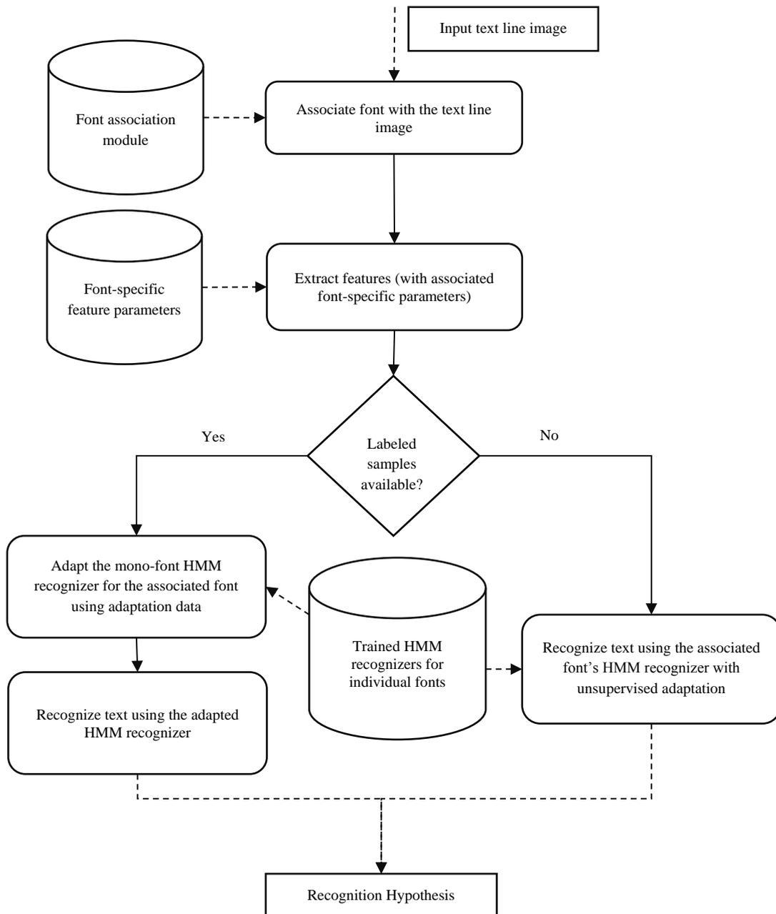
Figure 6.1: Framework for machine printed text recognition. (Figure adapted from (Ahmad, Mahmoud, and Fink 2016))
