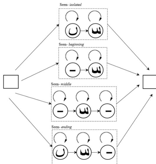
Figure 5.4: An illustration of constructing character models using sub-character HMMs. (Figure adapted from (Ahmad et al. 2013))
