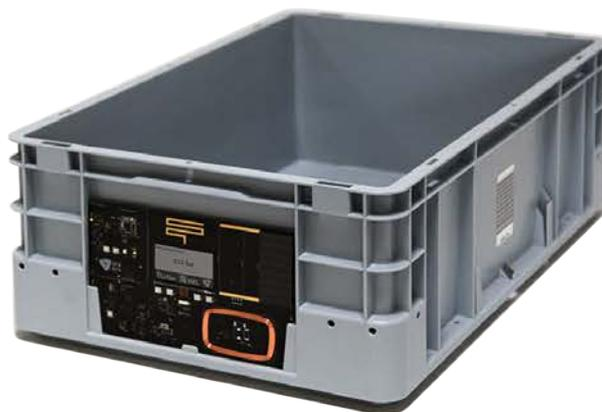
Figure 1: inBin: an energy-neutral IoT device for the materials handling application
