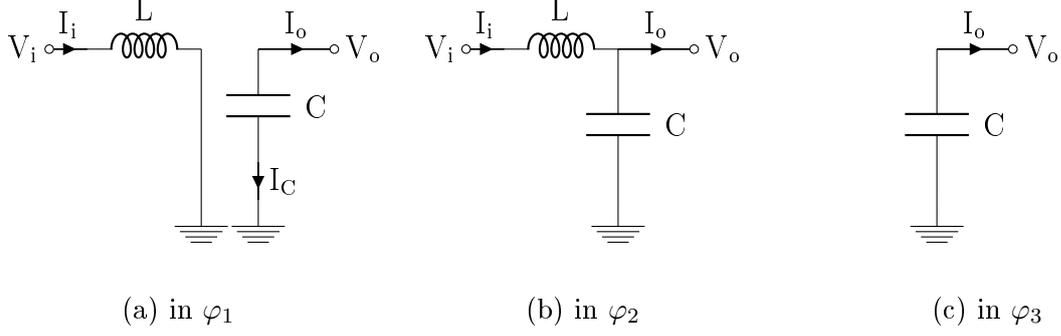
Figure 6: Boost converter circuit in each operational phase
