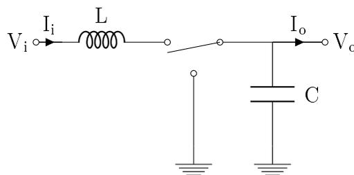
Figure 3: An ideal one switch boost converter
