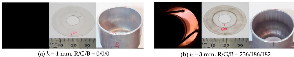
**Figure 13.** Long time exposures of the process glare, first plastic disc and flyer tube after MPW experiments at the Bmax setup ( $p = 0.1 \text{ mbar}$ ,  $\alpha = 0^\circ$ ,  $g = 1.5 \text{ mm}$ ,  $E = 4.5 \text{ kJ}$ ,  $I_{\text{max}} = 365 \text{ kA}$ ,  $\varnothing \text{ coil} = 41 \text{ mm}$ ,  $w_c = 10 \text{ mm}$ ,  $l_w = 6 \text{ mm}$ ): (a)  $l_c = 1 \text{ mm}$  (b)  $l_c = 3 \text{ mm}$ .
