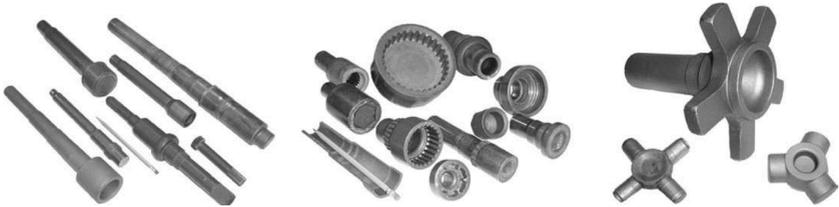
**Figure 2.22:** Parts produced by cold forging process combinations (Semiatin, 2005)
