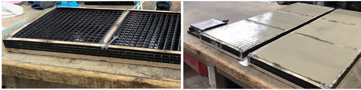
Fig. 4. Aspects of preparation of TRC panels and material testing prisms.
