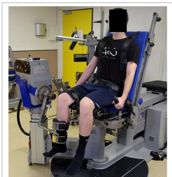
FIGURE 4 | Set-up of the IsoMed 2000 dynamometer and participant positioning for the knee strength testing.
