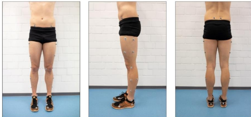
Figure 4. Lower-body marker set-up used for 3D motion analysis.
