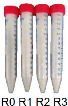
Figure 8. Photo of l -C 12 -DME product crystals purified by gassing crystallization, filtration, and washing after reaction with X = 80\% .
