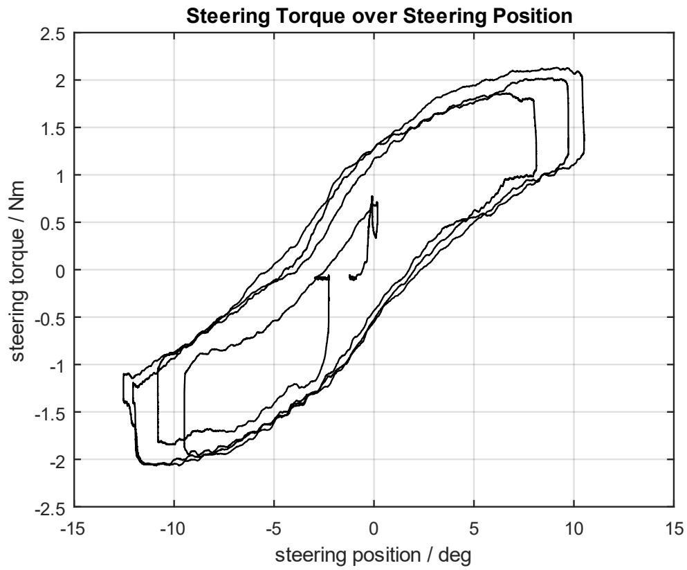
Figure 69: Performance Measurement – Cooperative Lateral Vehicle Guidance Control: Consistency and Symmetry of the Torque Build-Up at 60 km/h
