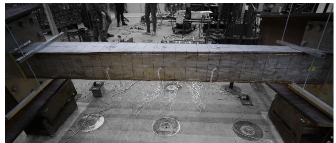
Figure 2: Shear test at a slenderness of \bar{\lambda}_w = 0.6
