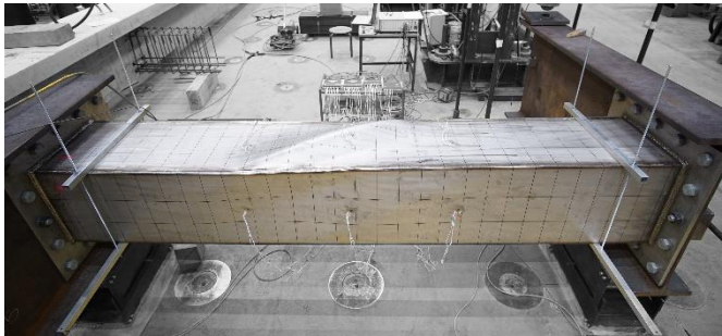
Figure 4: Typical shear buckling failure at a slenderness of \bar{\lambda}_w = 1,0 for hollow section 450-8-04-44
