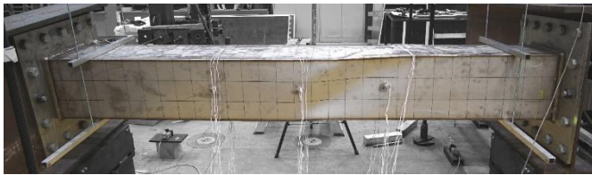
Figure 3: Typical shear buckling failure at a slenderness of \bar{\lambda}_w = 0,8 for hollow section 360-8-03-41
