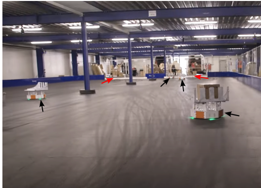
(a) Parcel sorting with the LoadRunner at the distribution center of DPD in Cologne [16]; 4 LoadRunner robots (black arrows) and 2 drop-off targets (red arrows) can be seen in the hall.
