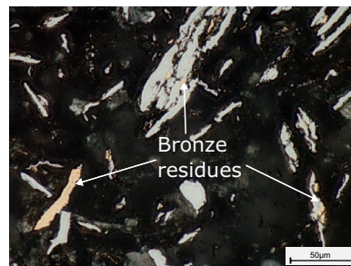
(a) Optical microscopy of mechanically alloyed powder with 300 rpm for 6 h
