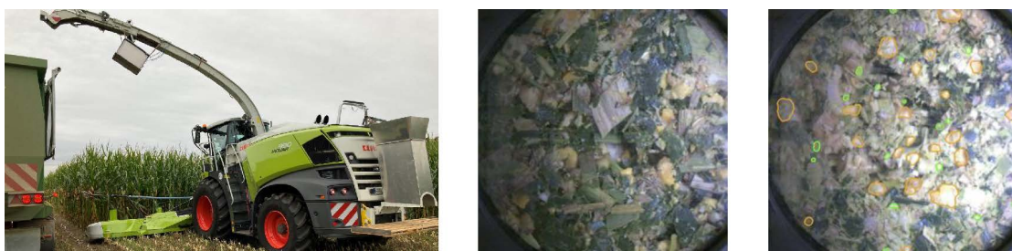
Figure 4.4: Harvest set up (left), example image captured during harvest (center) and its segmented version (right).
