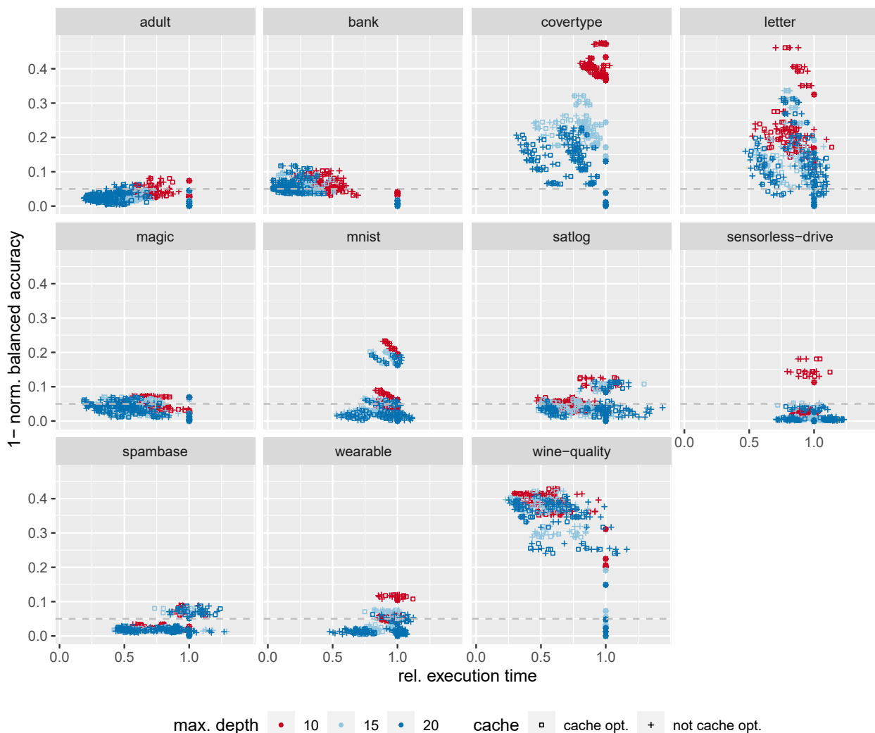
Figure 2. Normalized balanced accuracy values (with respect to the maximum value within each data set) and relative execution times for all data sets with different tree depths and separated by cache optimization or not.
