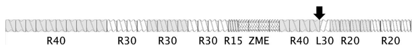
FIGURE 9 Optimal screw geometry for the Leistritz 27 mm Maxx extruder for the production of the three different hydrophobically ethoxylated urethane products. Indicated by the arrow is the feeding position of the alcohol.
