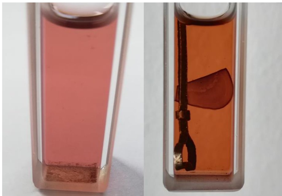
Figure 4.18 Cuvettes filled with the reaction mixture and the native (left) or immobilized HRP (right) after reaction times of 150 min at RT.
