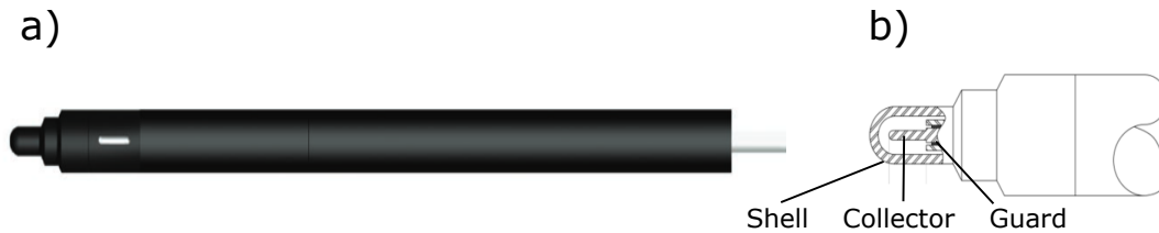
Figure 3.4: a) Photo of the EXRADIN T1 ionization chamber [122]. b) Technical drawing of the miniature Shonka IC [123].
