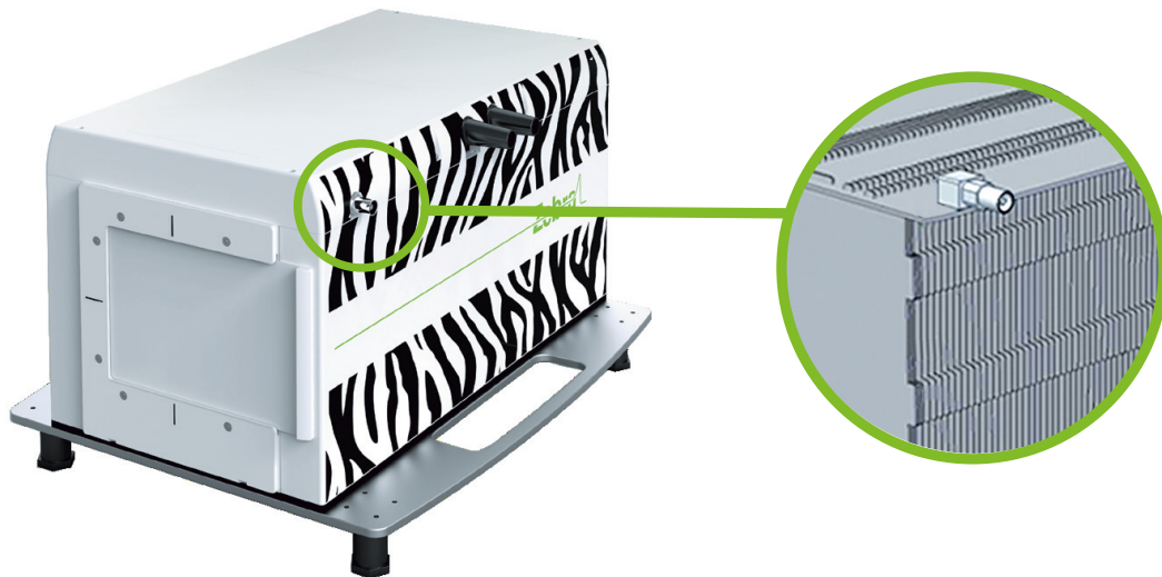
Figure 3.3: The IBA multi-layer ionization chamber (MLIC) Zebra detector is an important and time-saving device to measure Bragg Peaks and spread-out Bragg Peaks in a single measurement. This is achieved by the construction of 180 stacked electrodes (reproduction according Ref. [120]).
