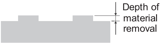
Fig. 2. Schematic illustration showing the method used to determine the material removal after the etching process.
