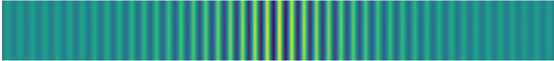
Figure 2: An eigenfunction in the strip for a combined medium with Neumann boundary conditions along all boundaries. The coordinates are x_1 and x_2 , the aspect ratio is changed in order to show x_1 from -45 to +45 . We see the interface mode, the eigenvalue \lambda = 8.03 is in the spectral gap of the media on the left and on the right, their geometry is generated with r_0 = 0.25 \pm 0.03 .
