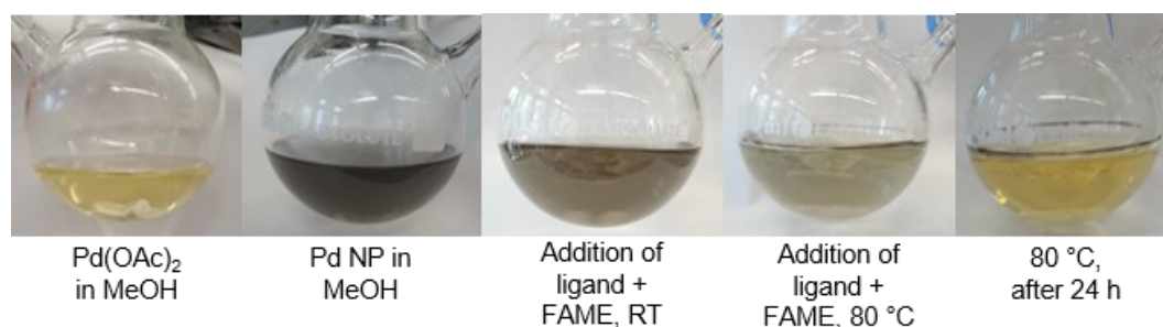
Figure 56: Evolution of the catalyst system throughout the reaction course. Reaction conditions: S:Pd = 1000:1, reflux, T = 80^{\circ}\text{C} , V_{\text{MeOH}} = 20 + 10 \text{ mL} , n_{\text{FAME}} = 16.9 \text{ mmol} ; L:Pd = 6, t_{\text{Preforming}} = 2 \text{ h} , t_{\text{complexation+reaction}} = 24 \text{ h} .
