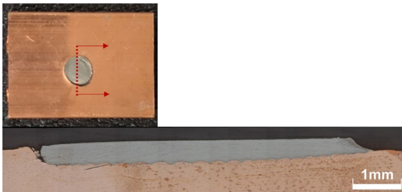
Figure 5: Cross sectional images of the Cu-Ti weld interface made with a 14° impact angle.
