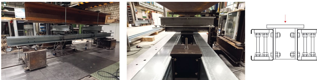
Fig. 12 Test setup of the four-point bending tests acc. to EN 15512 and detail of the load application for C-shaped sections
