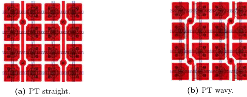
Figure 3.31: Sketches of the sensor design for a pixel pitch of 50\ \mu\text{m} \times 50\ \mu\text{m} with a (a) straight and (b) wavy punch-through design [83].
