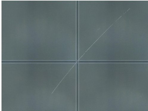
(a) Scratch, visible by eye, 20x magnification.
