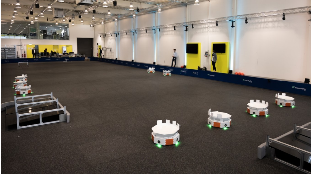
Figure 4.9.: Experimental setup at Fraunhofer IML [150]. The PACE Lab is equipped with a large-scale motion capture system to track robots and accurately evaluate their sim-to-real gap.
