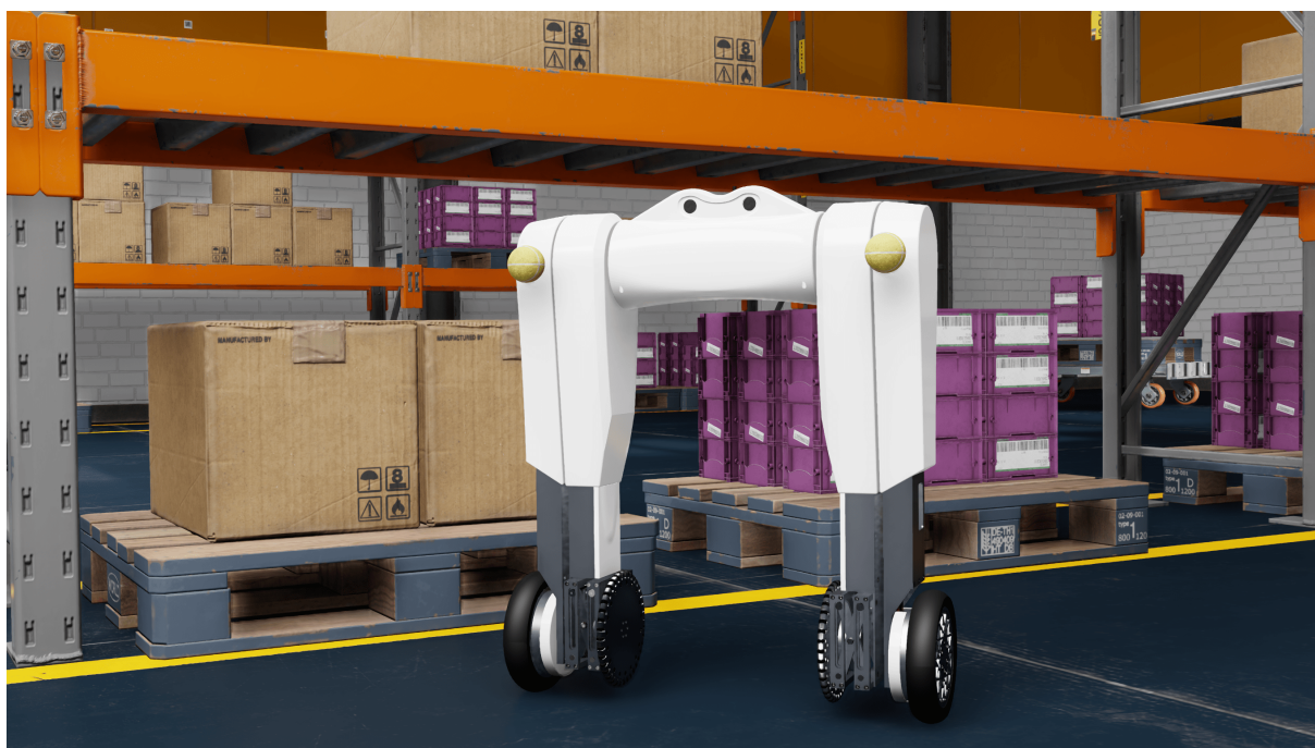
Figure 4.2.: evoBOT simulation model in NVIDIA Isaac SIM (based on prior publication [99]). Available in the state-of-the-art framework and via the Open Logistics Foundation repository 1 .
