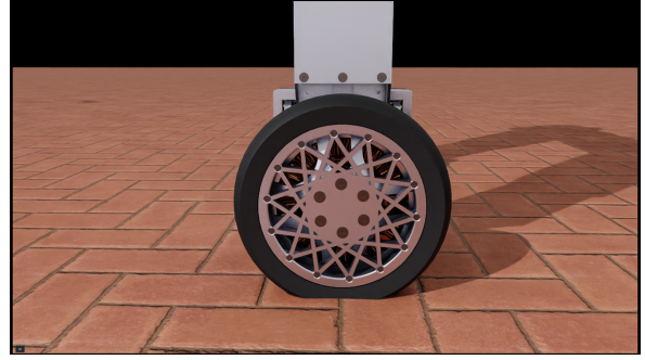
(b) Compliant contacts active, resulting in a contact surface between the wheel and the ground.
