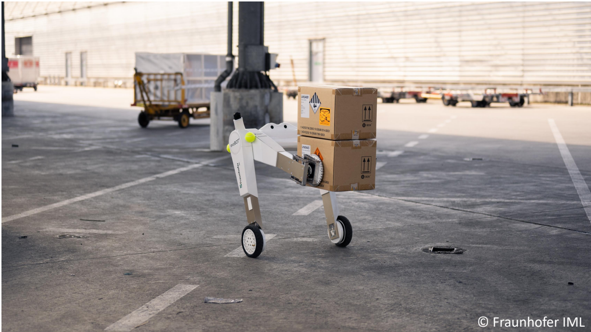
Figure 1.1.: evoBOT developed by Fraunhofer IML. A highly dynamic and flexible two-wheeled robot used as case study for learning-based control of challenging systems within this thesis [62].
