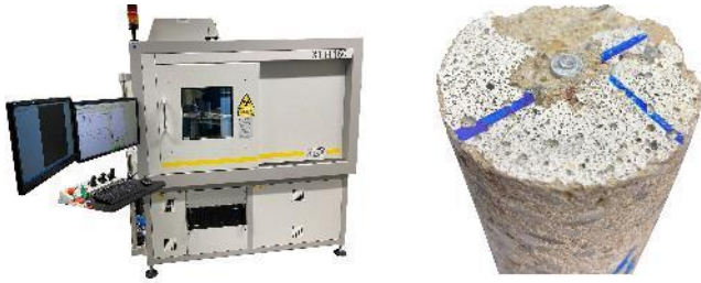
Figure 6 Computer tomography system and specimen.
