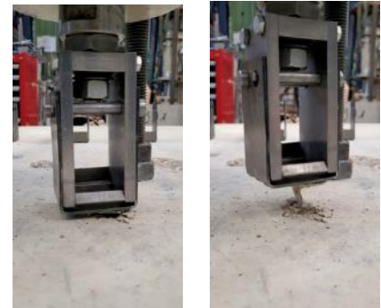
Figure 5 Installation set-up, using nail with light steel pull-out adapter and power actuated tool (top); Test configuration of pull-out test in two phases (bottom), indicating spalling at installation and bend nail at pull-out.
