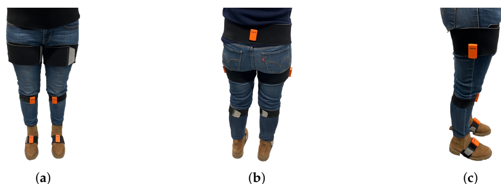
Figure 2. Sensor placement of the seven-sensor lower-body Xsens Awinda configuration. (a) Frontal view, (b) posterior view, and (c) lateral view showing sensors attached to the pelvis, both upper legs, both lower legs, and both feet.
