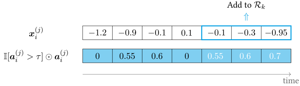
Figure 3.1.: Illustration of how to extract the most salient subsequences from the window \mathbf{x}_i^{(j)} (top) given the PGSM explanation \mathbf{a}_i^{(j)} (bottom). First, notice that we use \tau = 0.5 to threshold the explanation, only retaining values which are highly important. Second, we find subsequences in the thresholded explanation that are longer or equal than 3 entries and extract the corresponding values from \mathbf{x}_i^{(j)} to add to the forecasters RoC \mathcal{R}_k .
