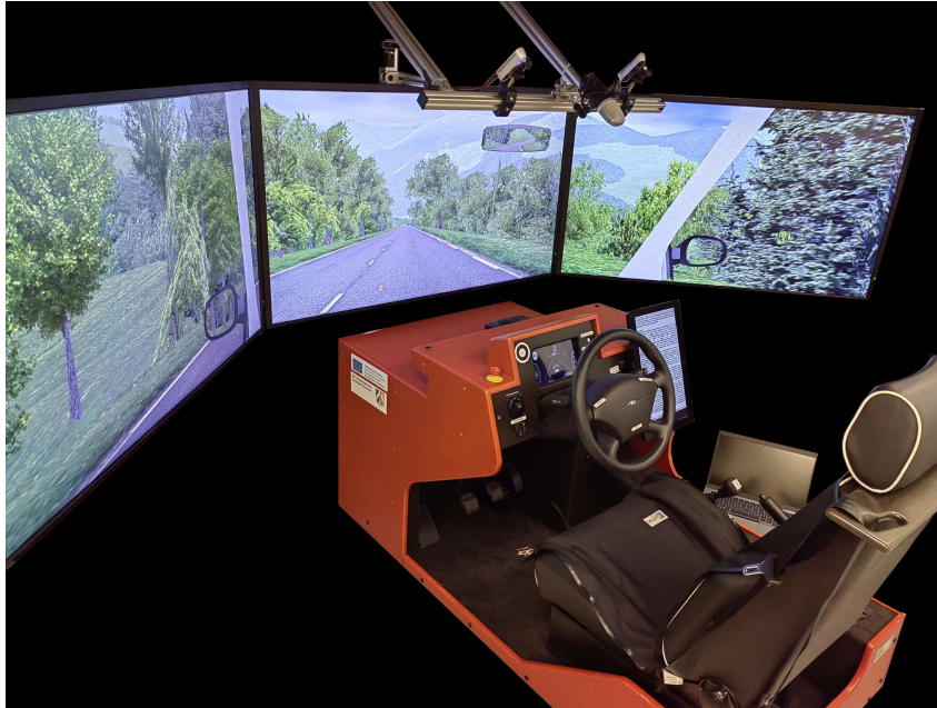
Figure C.1.: Static driving simulator employed to collect the manD 1.0 dataset
