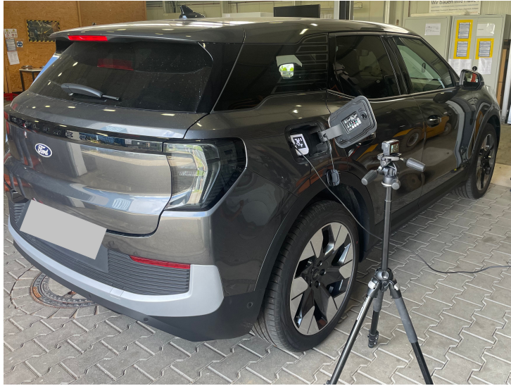
Figure 1: Experimental setup showing the positioning of the camera system and AprilTag marker on a Ford Explorer.
