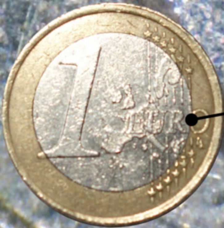
Figure 1.19: Coin — The 1 € coin is composed of an inner copper-nickel circle and an outer nickel brass ring. Over eight billion 1 € coins circulated as of 2022, which is 5.6 % of all € coins by quantity or 24.8% by value [78].
