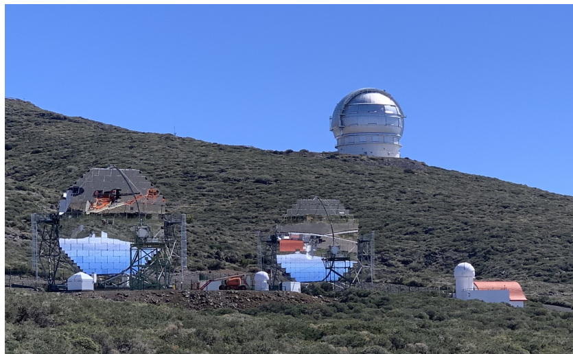
Figure 2.7: The MAGIC telescopes on La Palma with M1 on the left, M2 in the center, and the counting house with the LIDAR dome on the right. The Gran Telescopio Canarias (GTC) can be seen in the background.
