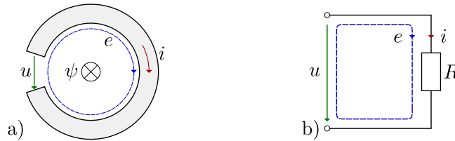
Figure B.2: Ring from Figure B.1 with one section removed: a) Cross-section, b) equivalent circuit. Now a voltage u can be measured at the open ends of the ring. The current i equals zero.
