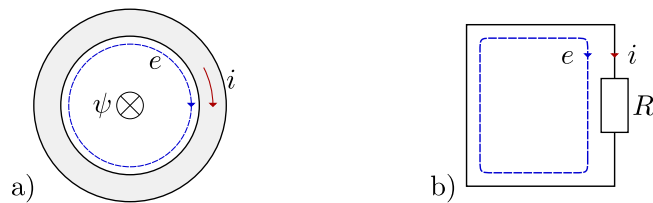
Figure B.1: Ring made of conductive material acting as a coil: a) Cross-section, b) equivalent circuit. The electromotive force e caused by the variation of \psi over time drives a current i .
