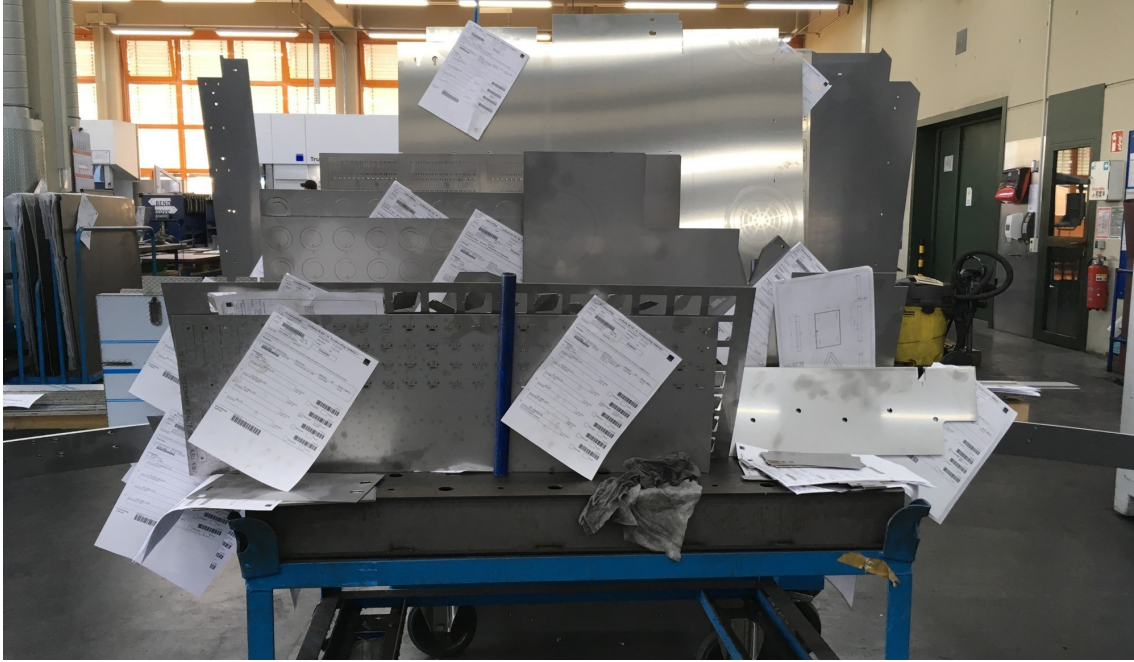
Figure 4.2: Work accompanying documents on sheet metal parts. Image courtesy of TRUMPF.
