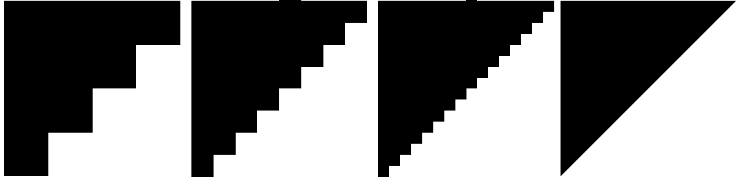
(a) Mesh size h = \frac{1}{4} : \text{TV}(u_h) = 1.5 . (b) Mesh size h = \frac{1}{8} : \text{TV}(u_h) = 1.75 . (c) Mesh size h = \frac{1}{16} : \text{TV}(u_h) = 1.875 . (d) Limit function u : \text{TV}(u) = \sqrt{2} .
